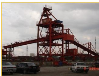
• Raw Material Yard Conveyor System & Transfer Station
