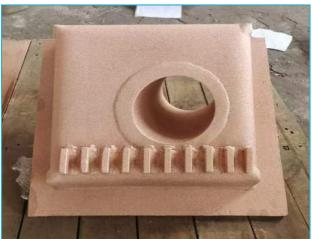
Copper contact pad for EAF and LF electrode arm
